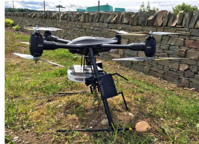
Source: I. B. Times, “Nokia and EE trial mobile base stations floating on drones to revolutionise rural 4G coverage,” url: <https://www.ibtimes.co.uk/nokia-ee-trial-mobile-base-stations-floating-drones-revolutionise-rural-4g-coverage-1575795>, 2016.
