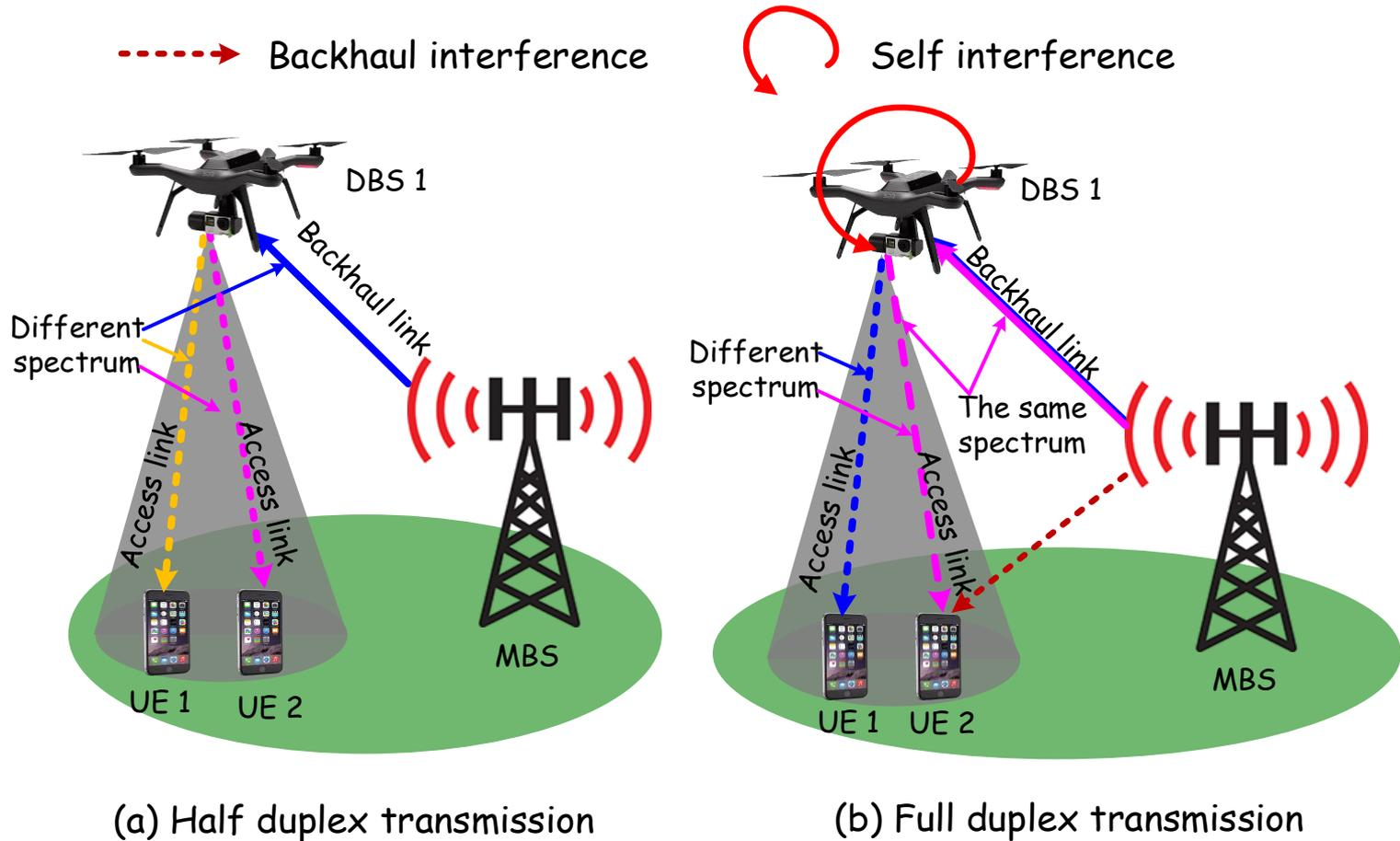
Fig. 1. DBS communications with half duplex and full duplex.
