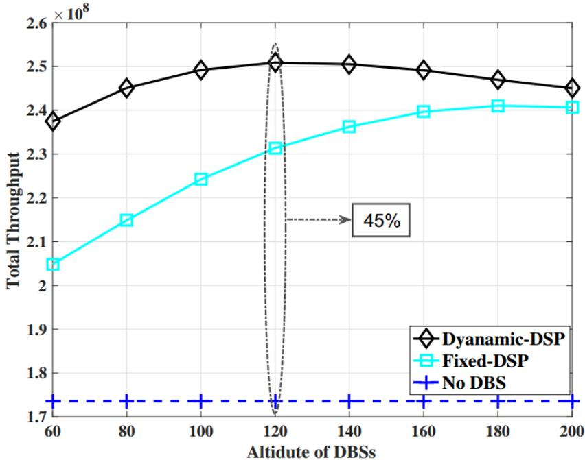
Fig. 6. Throughput versus altitude.
