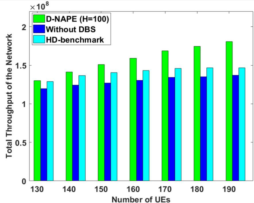
Fig. 3. Throughput versus the number of UEs ( $H=100$ ).
