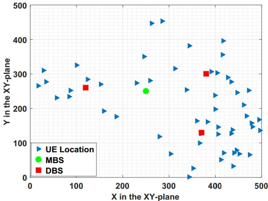
Fig. 8. DBS placement by Dynamic-DSP.
