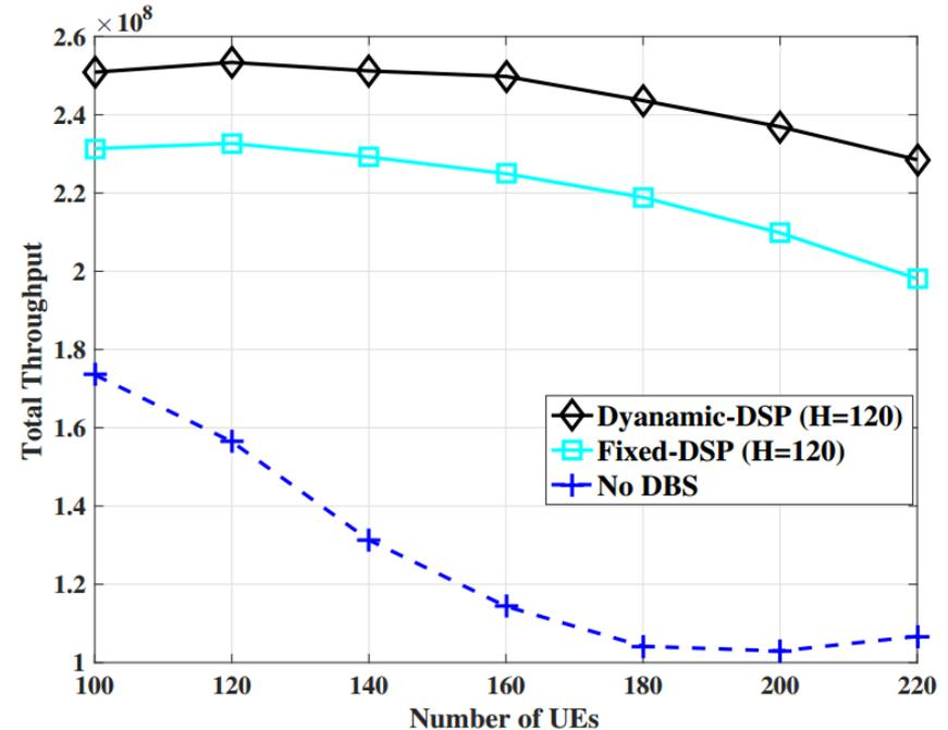
Fig. 7. Throughput versus the number of UEs.
