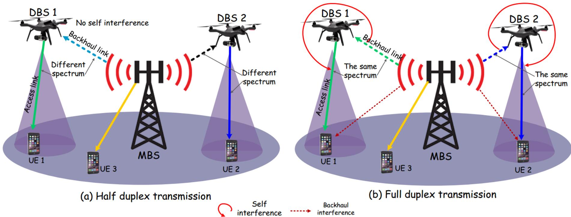
Fig. 4. Full duplex and half duplex communications with DBSs.
